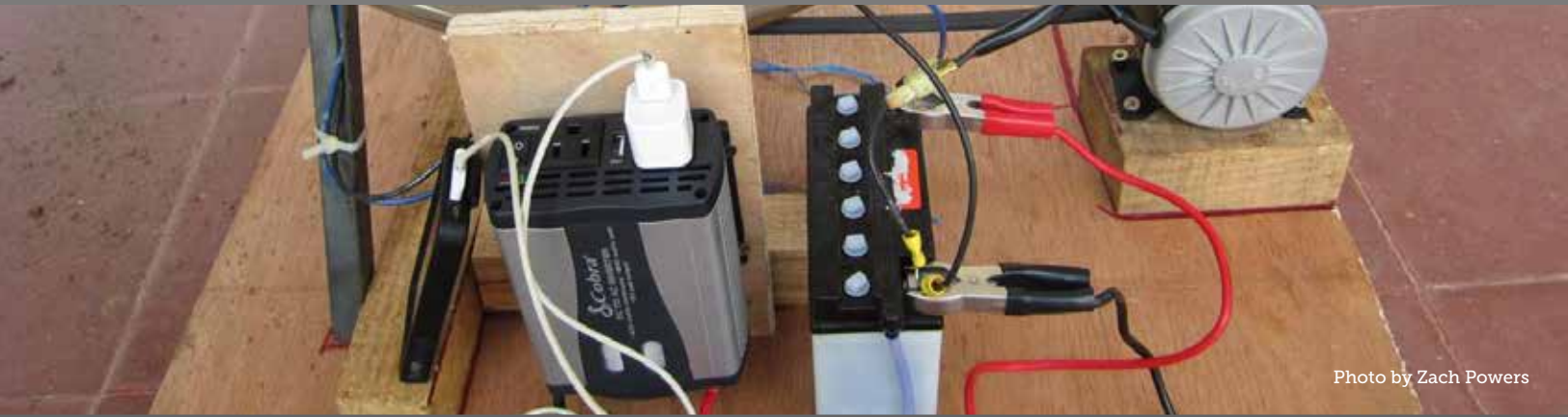
"Bici-generadora" - a student designed and built bike-powered generator
