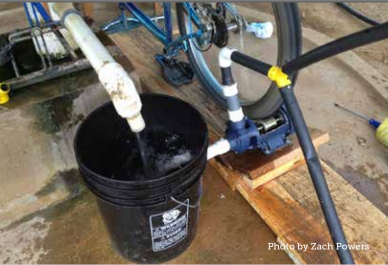
"Bici-Bomba" - a student designed and built bike-powered water pump
